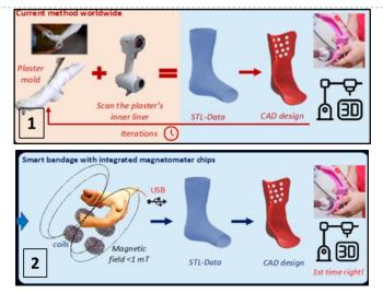
Workflow for current orthoses design (1) vs. future workflow with the smart bandage (2)
